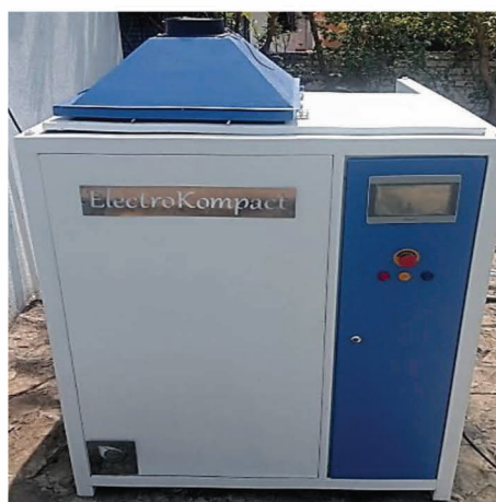
ElectroKompact : Combined Process of Electrocoagulation and Electrodialysis
